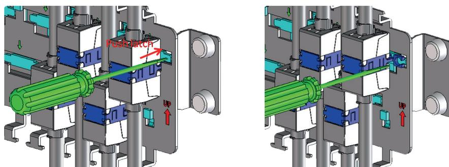
Push the plastic latch with a screwdriver to inside and slide the coupler on the corresponding side upwards.
